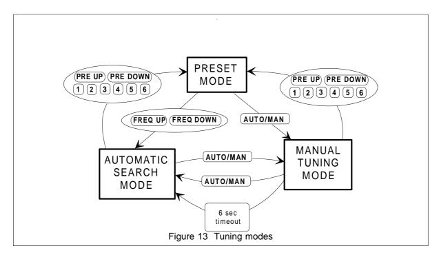
In search tuning mode, after pressing the FREQ-UP / FREQ-DOWN key, the frequency starts running and will stop on either a new frequency or at the frequency from which the search was started. For this search action two criteria are taken into account:
