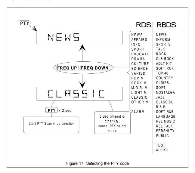
PTY codes "ALARM" / "TEST" / "ALERT!" can not be selected. The radio will respond to a PTY alarm message in the same way as a TA traffic announcement, independent of TA mode. For the USA application the RBDS PTY table is used.
