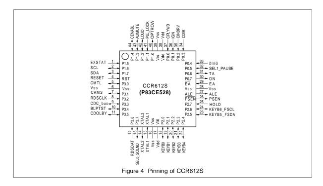
In case of conventional audio sound control circuitry, pin SEL0\_SOLND and SEL1\_PAUSE are used to select between the various audio sources (radio, CD-changer, cassette, external output) by means of a dual 4 channel analogue multiplexer (e.g. HEF4052B). If a TEA632x is installed these pins can be used for respectively solenoid control and AMS pause input control.
