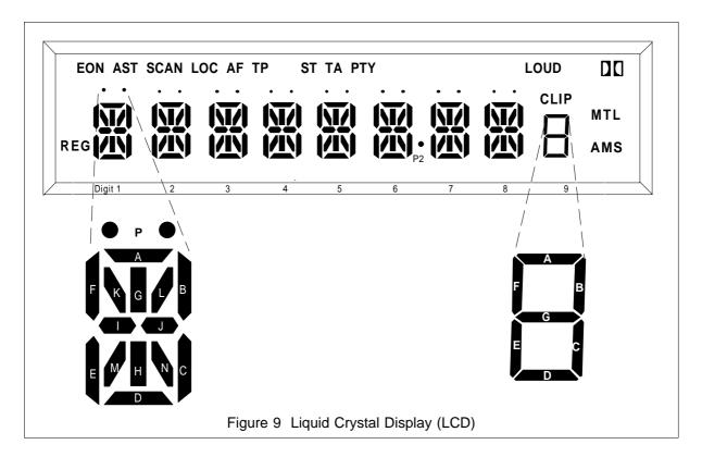
The 143 segment display is driven by one PCF8576 operating in 1:4 multiplex mode (4 backplanes BP0, BP1, BP2 and BP3) and a 1/4 (4 levels) LCD bias configuration.
